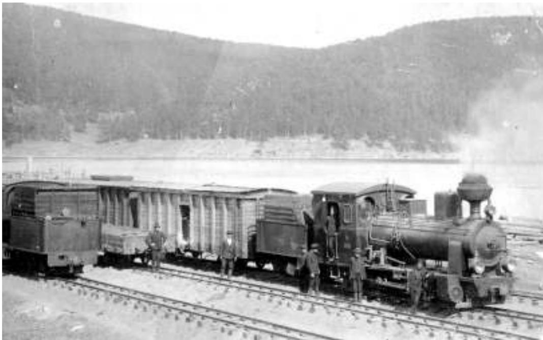
A Koppel 0-8-0 on the Beloretzk system in the Southern Urals, c.1914. (The covered van behind the loco is a special tank wagon for some kind of alcohol. It was common in Russia to build alcohol tanks inside covered vans for better protection from theft).
